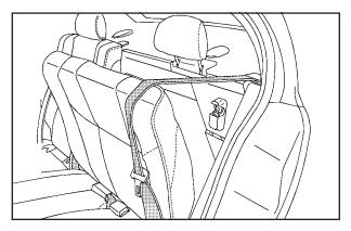
Once the handle is pulled, the seatback can be pushed open through the trunk, or pulled open from the inside of the vehicle.
